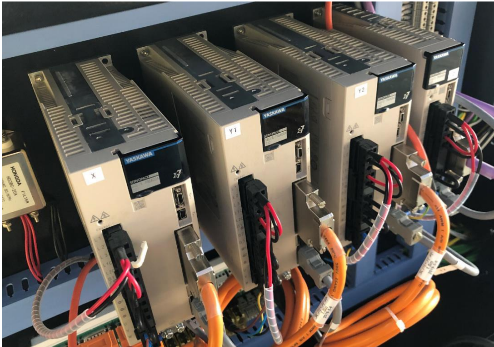
Az alkalmazott servo motorok Schneider servo motors and drivers. X, Y1, Y2: Schneider 1000W. Z: Schneider 400W. Motor reducer is SHIMPO.
