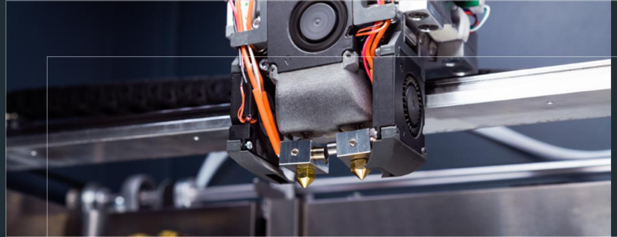
The Zmorph's advanced full metal Dual Drive Dual Extruder can heat up to 300°C. Waste Remover for wiped waste, matched with Tripple Control System on a filament flow keeps interrupted, high-quality, repeatable 3D printing for the most demanding applications.
